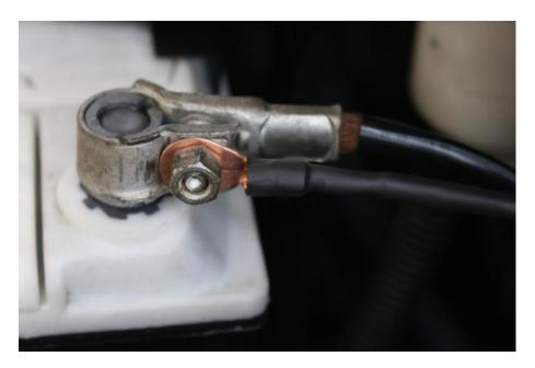
The sensor is connected to the battery's negative terminal, where the temperature can be most accurately measured.
