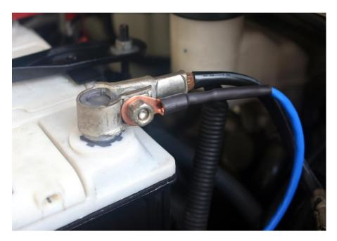
In the image above you can see how the sensor is installed on the negative terminal of the car battery by first removing the nut from the battery terminal inserting the sensor connector onto the bolt of the battery terminal connector, then installing the nut back onto the terminal bolt.
